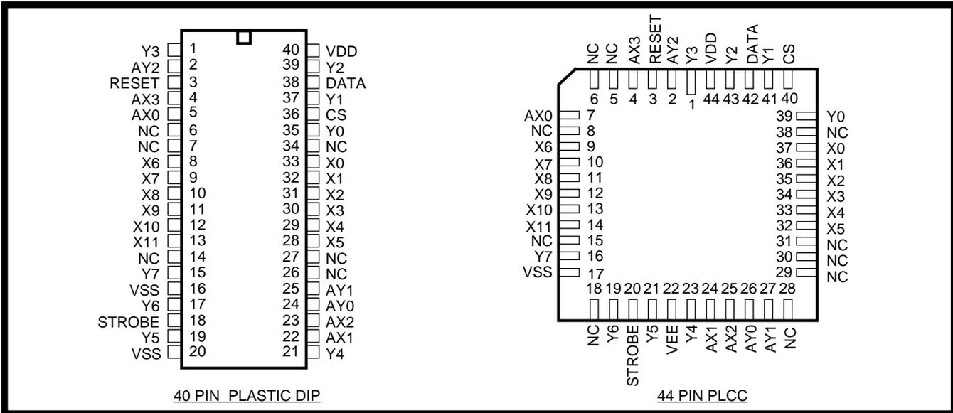
Figure 2 - Pin Connections
